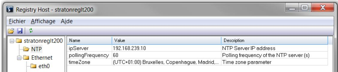
NTP Settings: By default the fields are empty, and the NTP function is not active.
