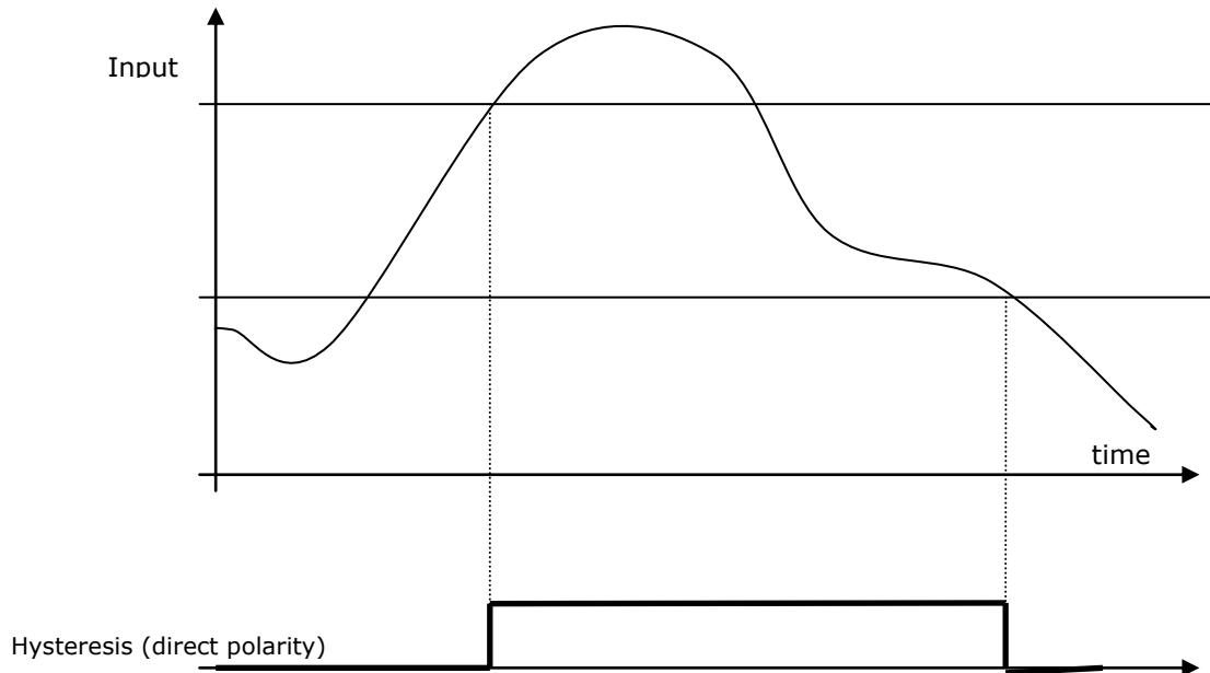
Parameters: set the high and low threshold. Choose the digital associated output.
