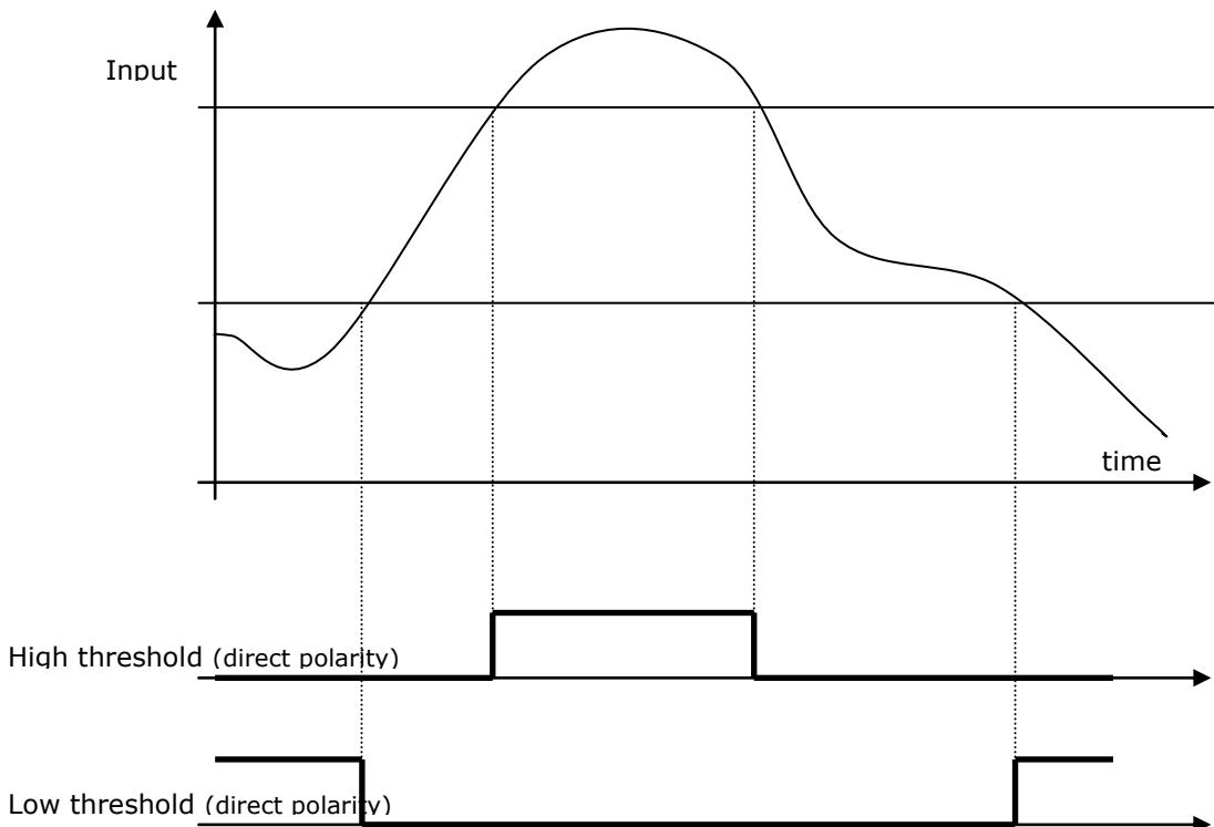
Parameters: set the high threshold value and its digital output associated. Set the low threshold and its digital output associated. The 2 outputs must be different.
